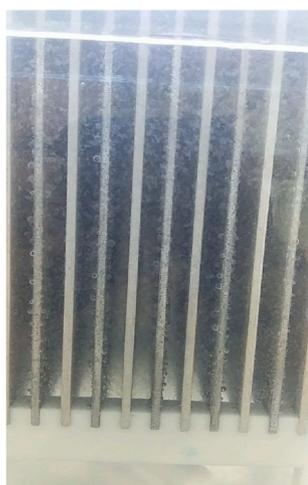
Fig. 9. A typical image of attached gas bubbles on the electrode surface in the conventional ECF (passive cathode).
