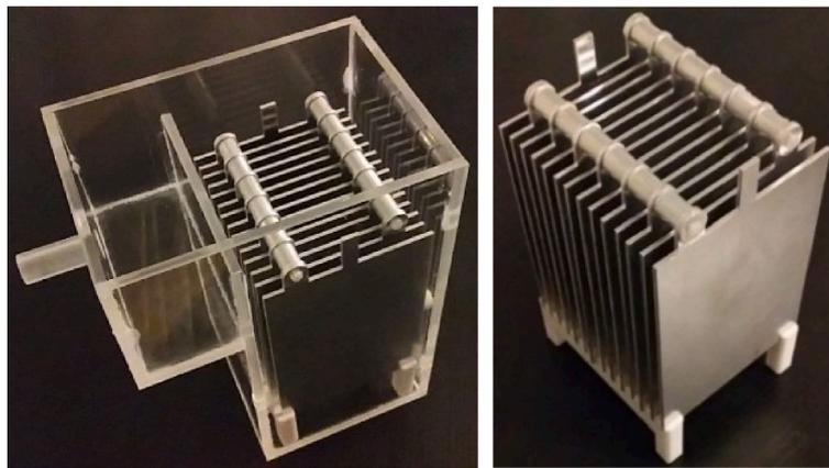
Fig. 1. Schematic and constructed rectangular cell configuration with plate electrodes.
